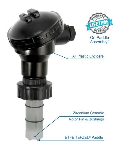
Simple to install with time-honored reliable performance, Truflo TIR Series Paddle wheel Flow Sensors are highly repeatable, rugged sensors that offer exceptional value with little or no maintenance. The TIR Series has a process-ready open collector signal with a wide dynamic flow range of 0.1 to 10 m/s (0.3 to 33ft/s). The sensor measures liquid flow rates in full pipes and can be used in low pressure systems.
